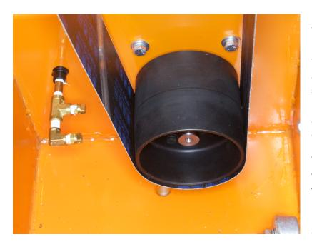
You'll see the double water sprayer in front of the lower roller in the water basin. This is the solenoid-activated water spray for the belt sander. It is activated when the power to the sander is turned on and de-activated when it is turned off from the power switch.
