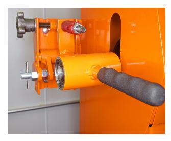
The most important part of your belt sander to get acquainted with is the arm assembly. This is located on the top left side of your new belt sander. The tensioner assembly consists of a black rubber handle that pulls down the upper roller to mount and un-mount your abrasive belts.
